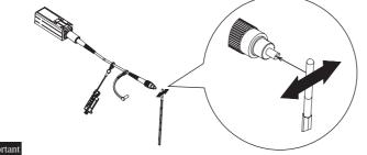
· The cleaner can only be used one time. Reusing the cleaner may result in dirt or scratches on the end surface, causing malfunctions or measurement errors. Discard after use. · Be sure to clean the fiber cleaner with the cloth for the cleaning part (white end face).
