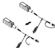
(2) Connect the fiber cable and calibration ROM with the Sensor Controller. Attach the fiber cable so that the projection of the fiber connector fits into the groove of the fiber adapter of the Sensor Controller. As pushing in the cable, turn the screwed region to the right.
