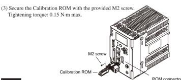
bushing in or pulling out the calibration ROM, be sure to turn off the power of the Sensor Controller. Otherwise, a failure might be caused
