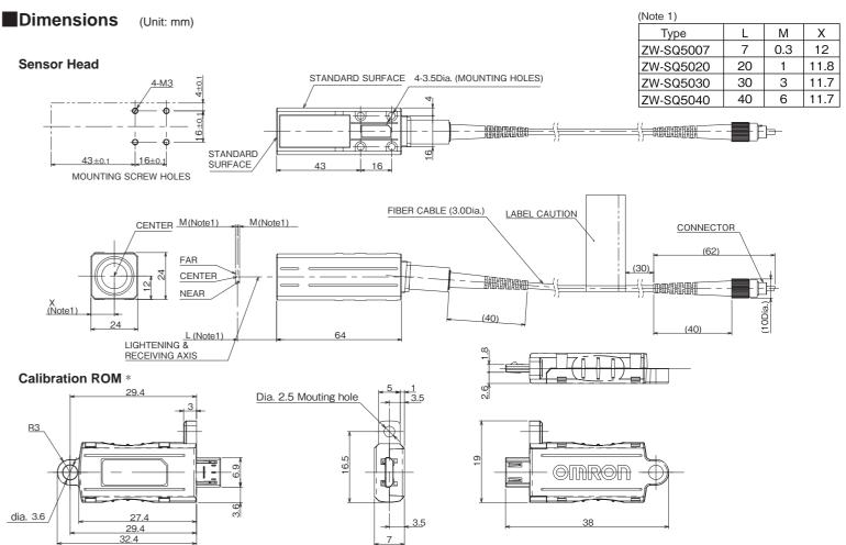
\* Included in the Sensor Head (ZW-SQ5007/SQ5020/SQ5030/SQ5040). Be sure to use the Sensor Head and Calibration ROM of the same serial numbers.
